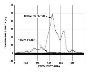
Figure 3. Effect of Filter on 100 mV Noise
