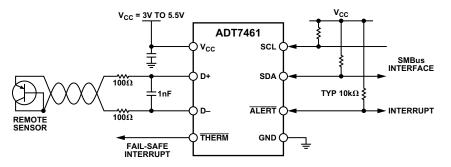
Figure 1. Circuit Diagram
